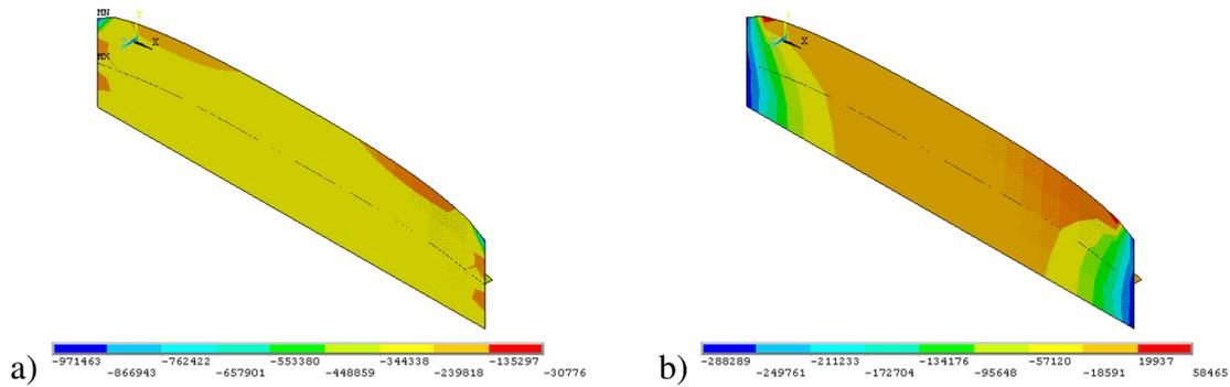
Fig. 8. Stress plot for the stiffened rectangular plate (a) X direction ( $\sigma_{xx}$ ), (b) Y direction ( $\sigma_{yy}$ )
