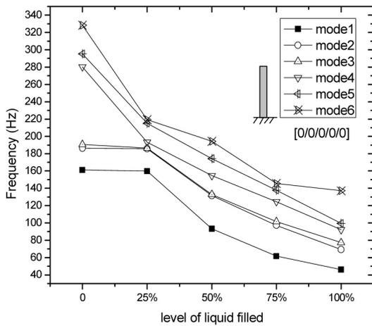
Fig. 18. Natural frequency variations with the level of liquid level for [0/0/0/0/0] lay up for CF box column
