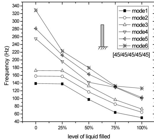
Fig. 19. Natural frequency variations with the level of liquid level for [45/45/45/45/45] lay up for CF box column
