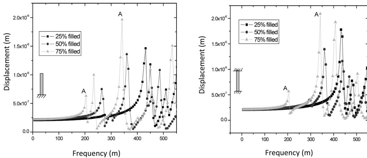
Fig. 16. Vibration responses at the excitation point for CF and CC box structure with 25 %, 50 % and 75 % liquid filled
