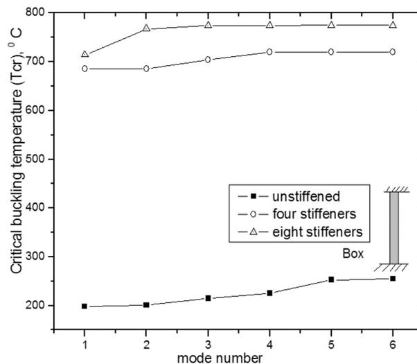
Fig. 4. Thermal buckling temperature of Box structures ( $L = 0.75 \text{ m}$ ) with and without internal stiffeners
