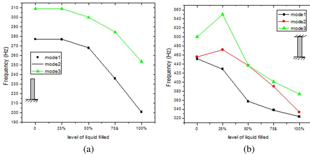
Fig. 12. Effect of fluid level in the container on the added mass frequencies (a) C-F and (b) C-C
