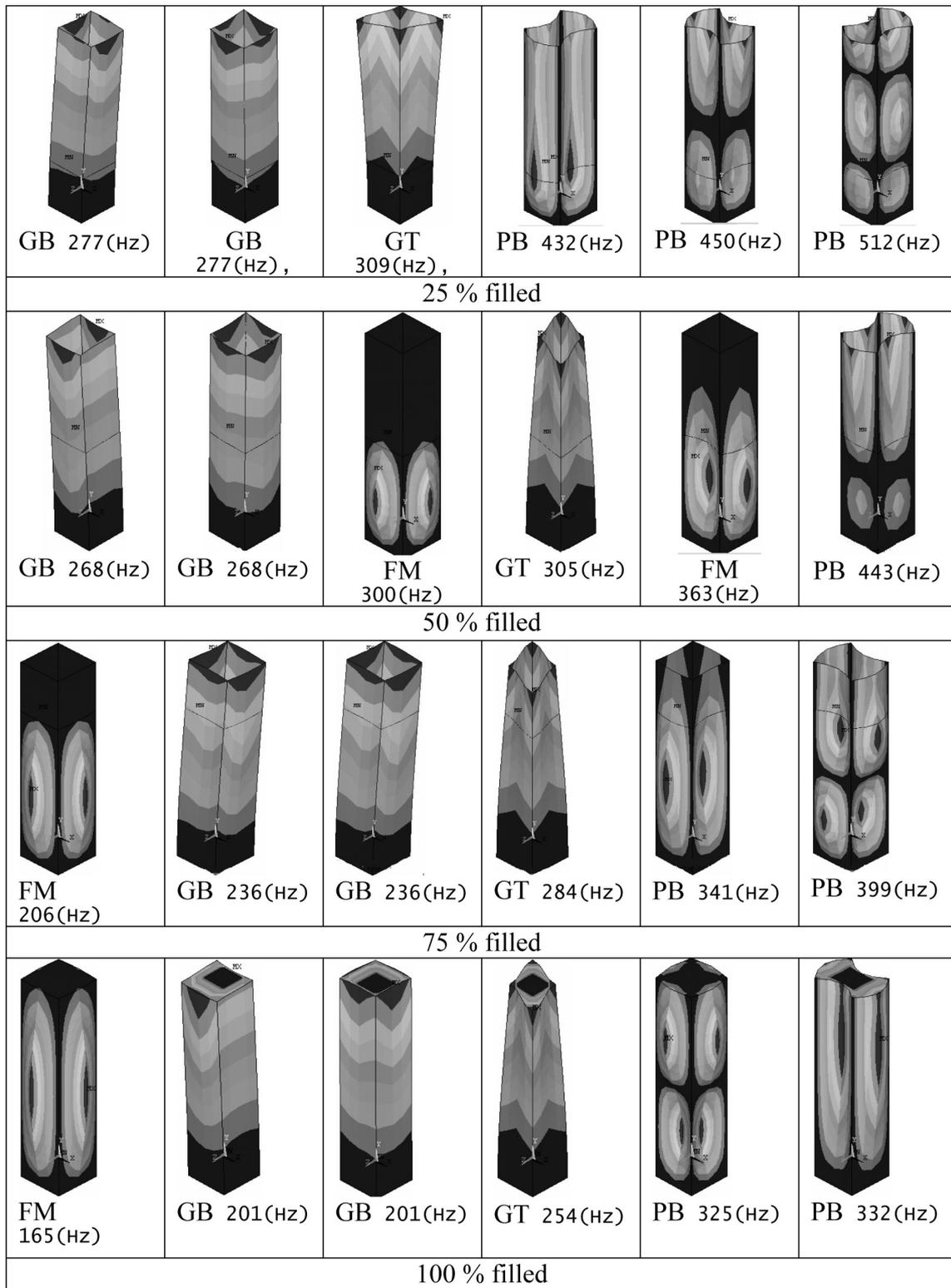
Fig. 13. First six mode shapes of CF box container filled with different level of liquid. (GB-Global bending mode; GT-Global twisting mode; FM- fluid dominating mode; PB-Plate bending mode)
