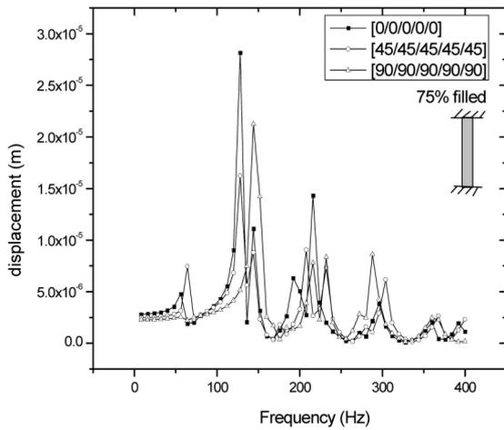
Fig. 27. Displacement at the excitation point for various values of fiber orientation for CC box column
