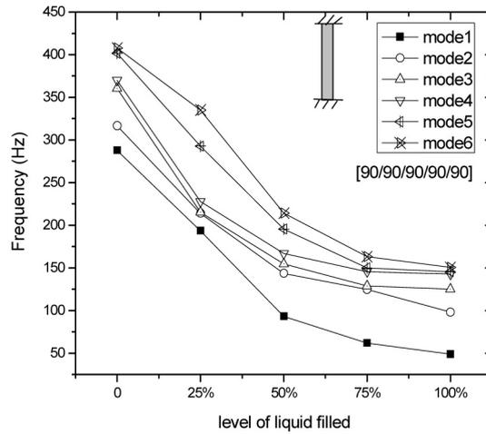
Fig. 24. (c) Natural frequency variations with the level of liquid level for [90/90/90/90/90] lay up for CC box column
