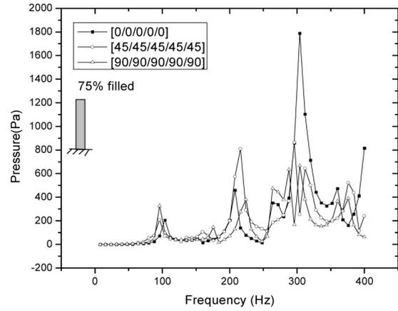
Fig. 26. Acoustic response various values of fiber orientation for CF box column
