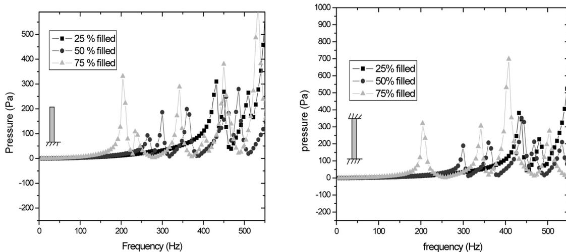
Fig. 17. Acoustic responses at the center of the acoustic cavity for CF and CC box structure with 25 %, 50 % and 75 % liquid filled
