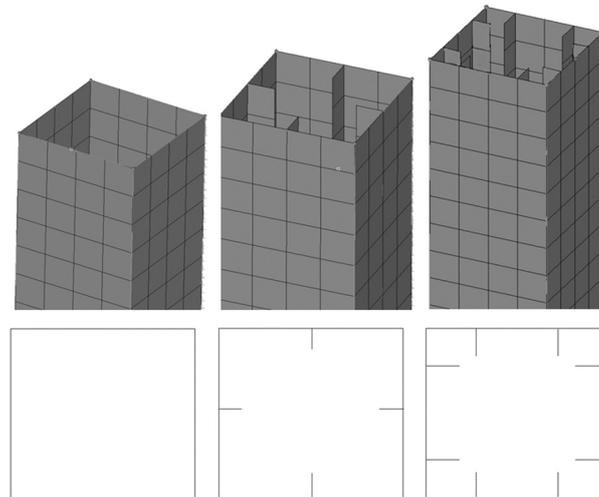
Fig. 2. Thin-walled structures with and without stiffeners
