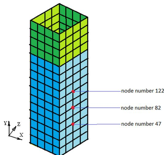
Fig. 15. Finite element model of rectangular box structure with 75 % fuel filled
