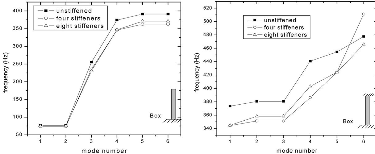
Fig. 7. Natural frequency of Box structures ( $L = 1.5$  m) with and without internal stiffeners
