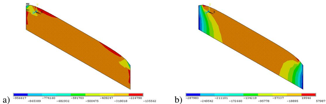
Fig. 9. Stress plot for the un-stiffened rectangular plate (a) X direction ( $\sigma_{xx}$ ), (b) Y direction ( $\sigma_{yy}$ )
