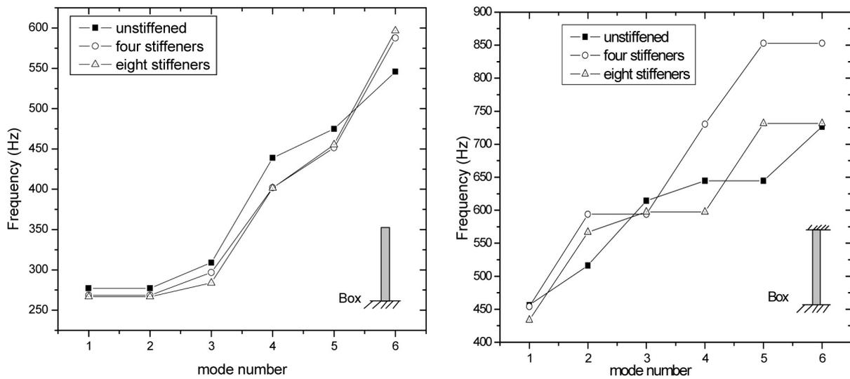
Fig. 6. Natural frequency of Box structures ( $L = 0.75$  m) with and without internal stiffeners
