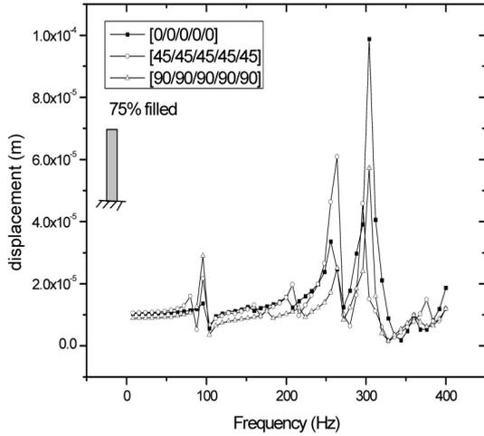
Fig. 25. Displacement at the excitation point for various values of fiber orientation for CF box column
