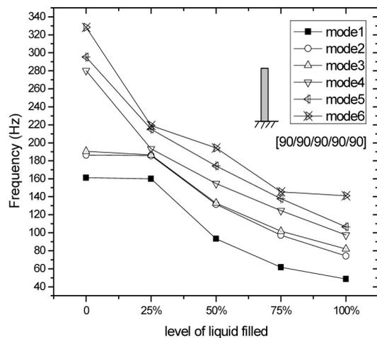
Fig. 21. Natural frequency variations with the level of liquid level for [90/90/90/90/90] lay up for CF box column
