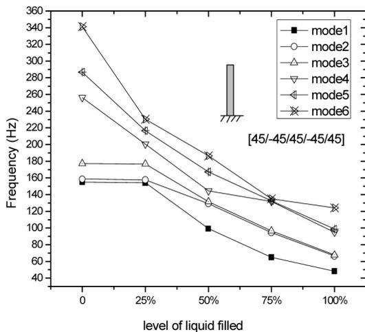
Fig. 20. Natural frequency variations with the level of liquid level for [45/-45/45/-45/45] lay up for CF box column
