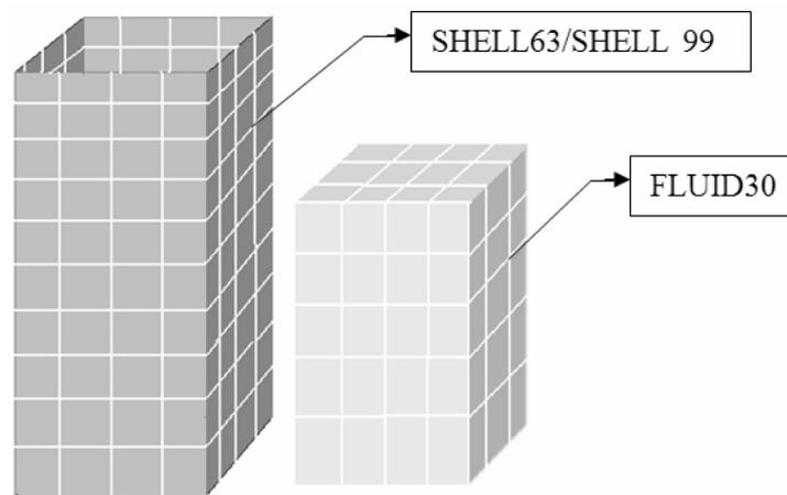
Fig. 10. FE model for structure and fluid
