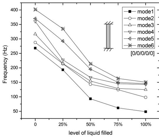
Fig. 22. (a) Natural frequency variations with the level of liquid level for [0/0/0/0/0] lay up for CC box column
