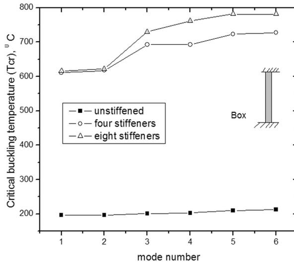
Fig. 5. Thermal buckling temperature of Box long structures ( $L = 1.5$  m) with and without internal stiffeners
