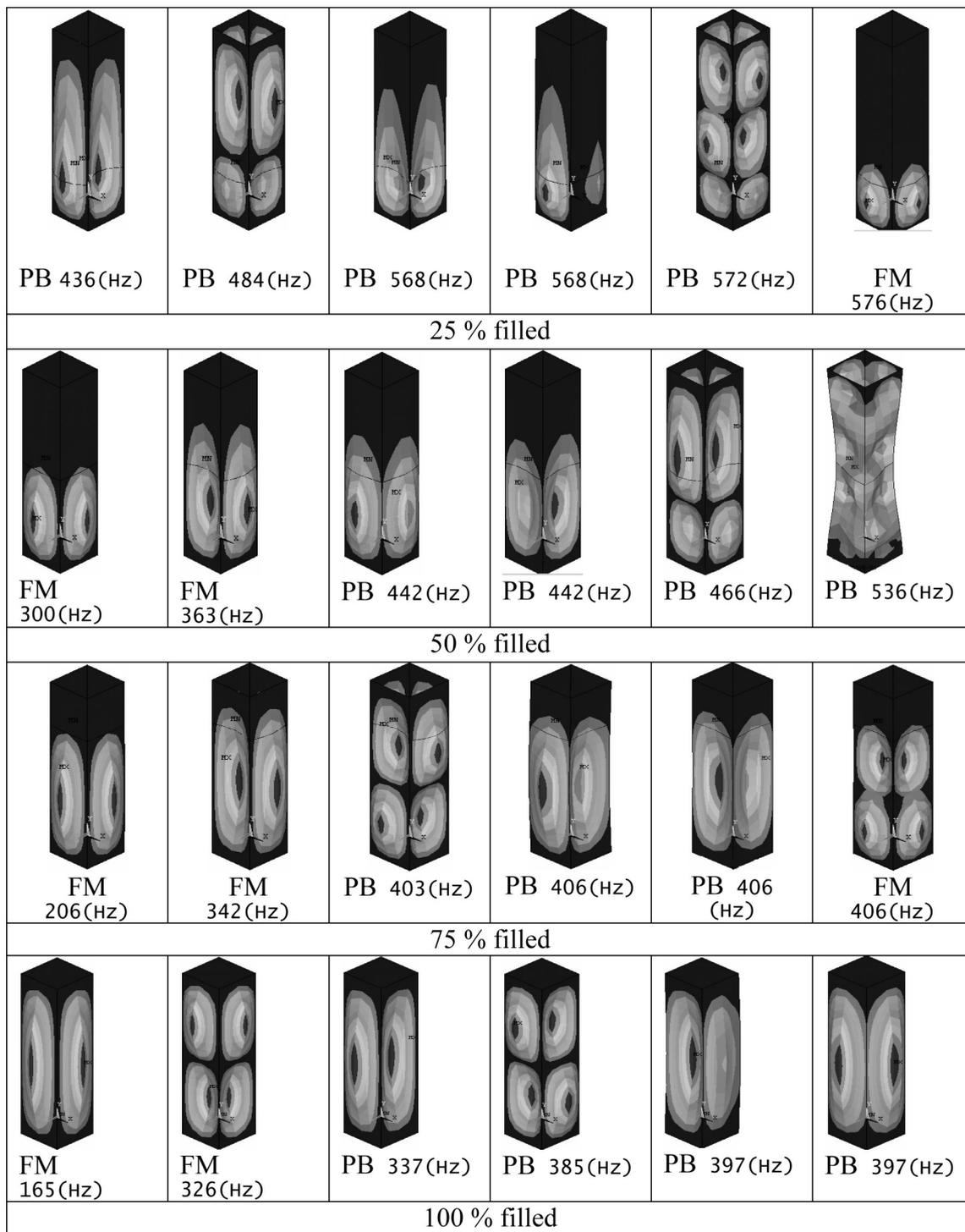
Fig. 14. First six mode shapes of CC box container filled with different level of liquid (GB-Global bending mode; GT-Global twisting mode; FM- fluid dominating mode; PB-Plate bending mode)
