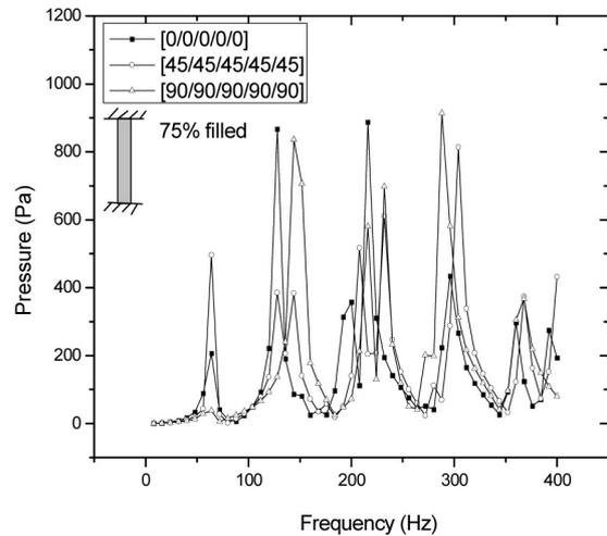
Fig. 28. Acoustic response various values of fiber orientation for CC box column
