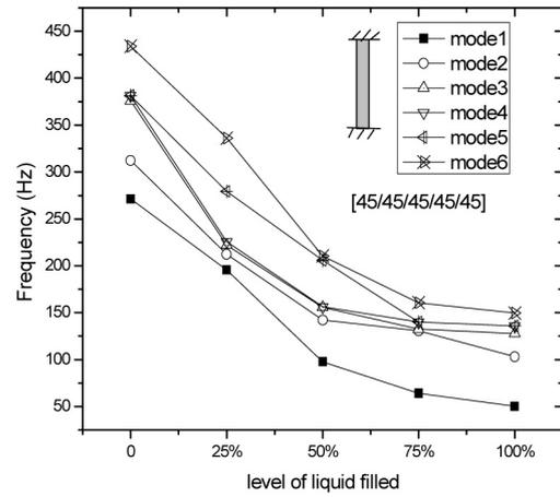
Fig. 23. (b) Natural frequency variations with the level of liquid level for [45/45/45/45/45] lay up for CC box column
