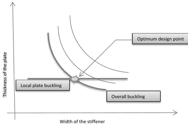
Fig. 1. Simplified optimum design curve for local and overall buckling
