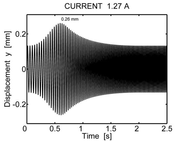
Fig. 11. Time history of the rotor displacement
