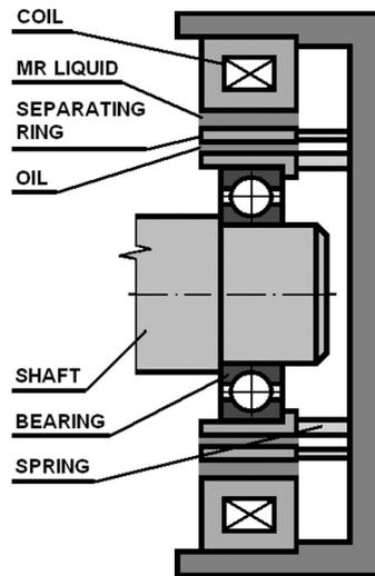
Fig. 4. Scheme of the damping device
