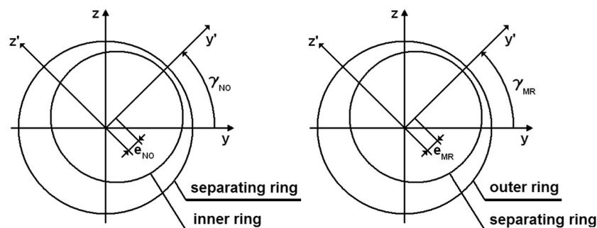
Fig. 5. The damper's coordinate systems
