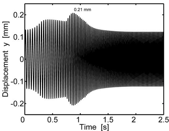
Fig. 22. Rotor displacement time history – variant 2
