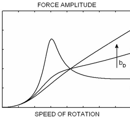
Fig. 2. Transmitted force – speed of rotation relationship
