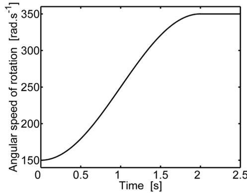
Fig. 7. Time history of required angular speed of the rotor rotation
