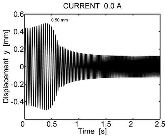
Fig. 10. Time history of the rotor displacement
