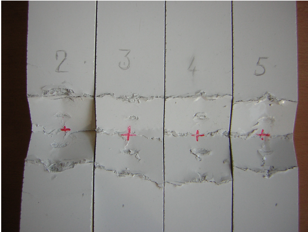
Fig. 6.36: Impact area on specimens after experiments.
