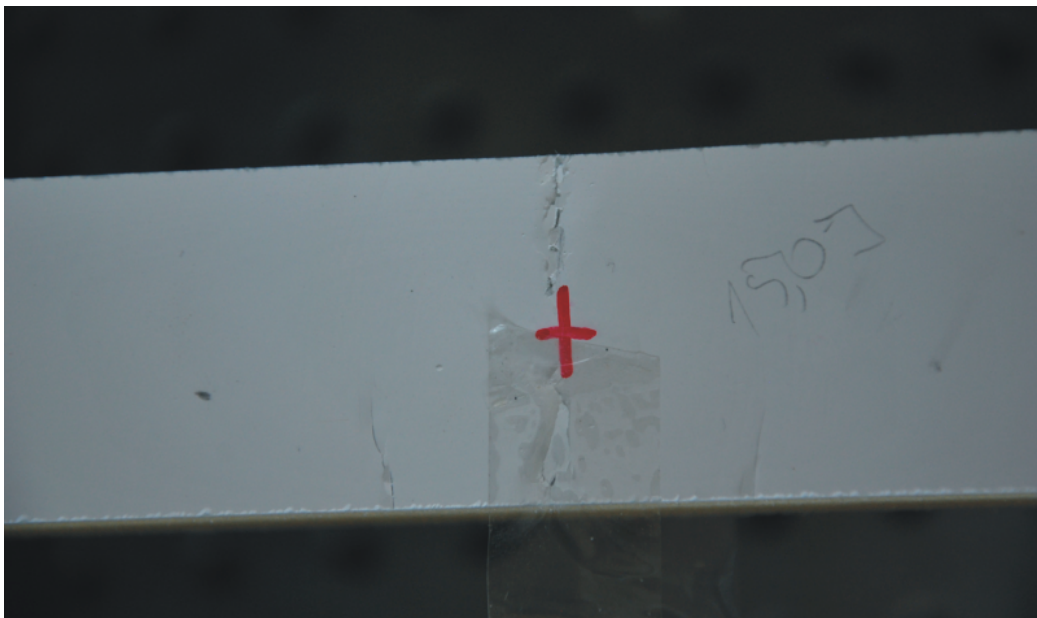
Fig. 6.24: Damage on the upper skin after the fourth impact on specimen no. 5.
