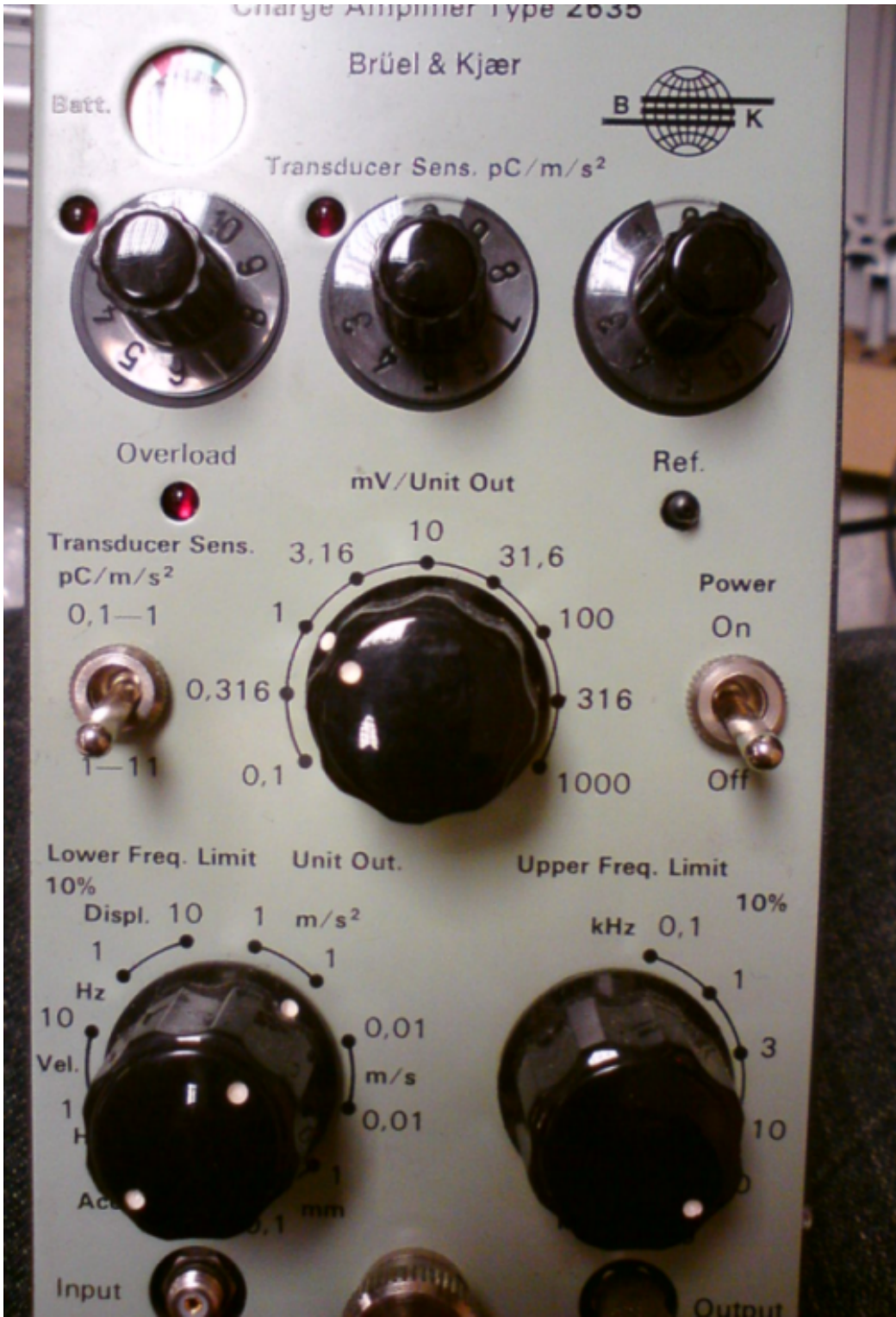
Fig. 5.15: Detail of charge amplifier front panel with settings.
