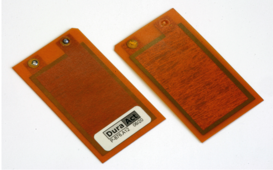
Fig. 4.12: Two piezoelectric patches P-876.A12 used in experiment.
