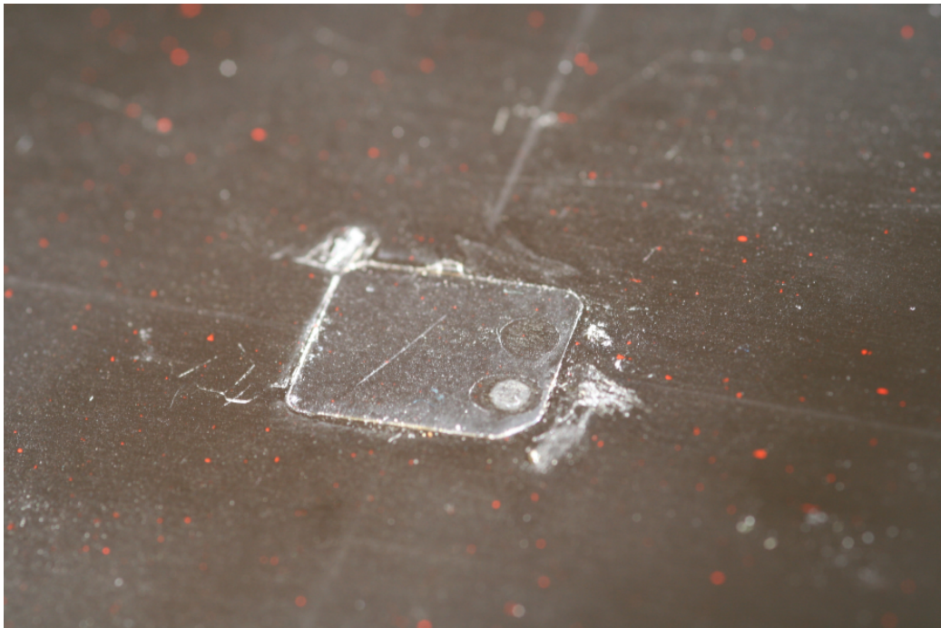
Fig. 6.14: Detail of area of unglued patch.
