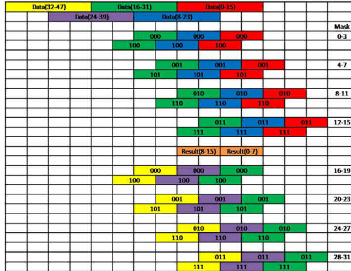
Figure 1. Computational arrangement for fast pattern matching. Data inboxes is the imm8 value
