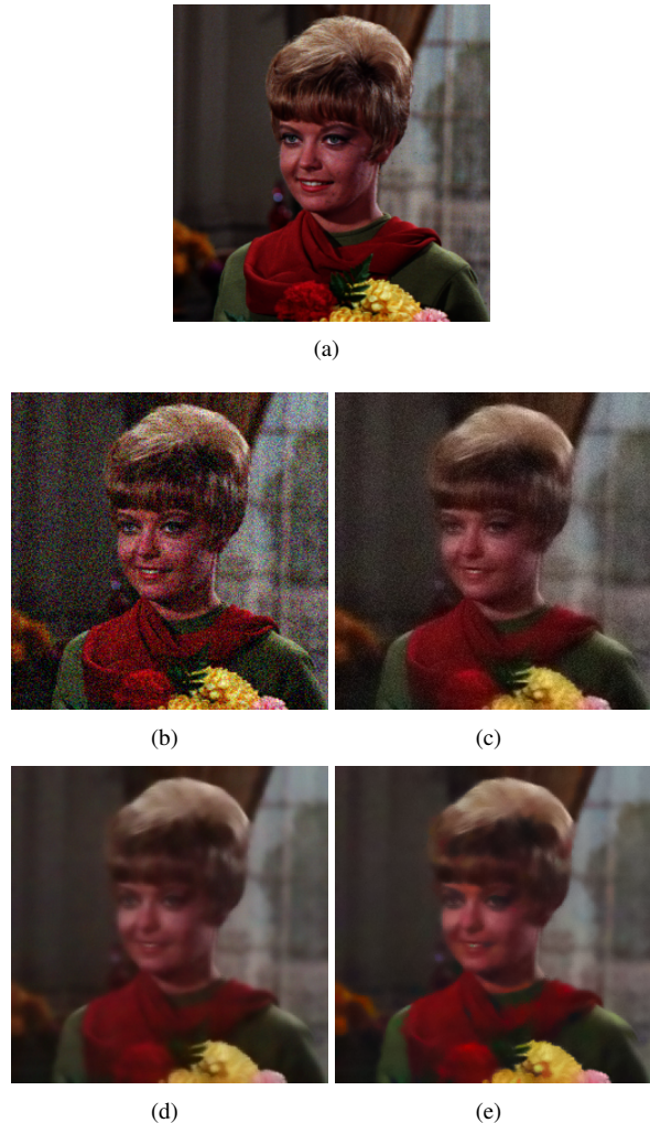
Figure 1: Denoising example. (a) shows the original image, (b) the image with Gaussian noise added to all RGB channels. (c) is the result using Neat Image at maximum filtering. (d) shows the denoising result using DenoiseMyImage. (e) is the result obtained using our algorithm. PSNR: (c) 26.69, (d) 26.35, (e) 27.20 ( \lambda = 5 )
