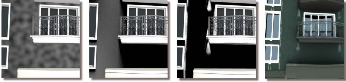
Figure 4: Summary of the method, from left to right: Porosity controlled by a noise texture – Computing rain accessibility rA – Computing strong flows and runs-out rfE – Computing reflectance modifications for final image.
