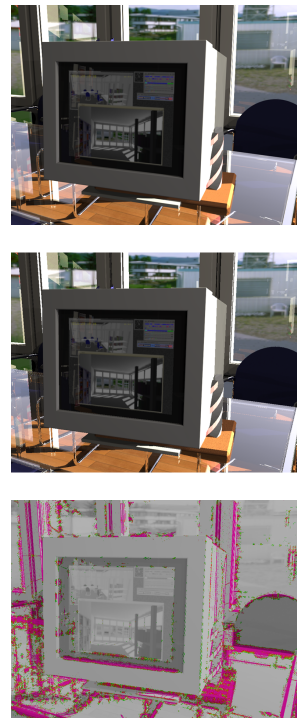
Figure 3: VDP comparison. Top: mask image; Middle: target image; Bottom: difference map with probability of detection - green:0-50%; yellow: 50-75%; red:75-95%; pink:95-100%
