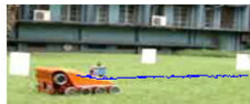
Figure 11a: Trajectory identified after rejecting outlier data using averaging window of 4\sigma gate
