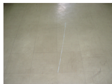
Figure 7: White mark in the center shows the path followed by the camera mounted on a trolley. The track line was created using a white marker while pushing the trolley at an approximate constant speed.
