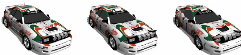
Figure 9. Racing car model. From left to right: original model (8345 triangles), model simplified to 66% (5506 triangles) and 33% (2753 triangles).
