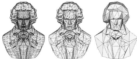
Figure 1: Three levels of detail of the Ludwig model. Left, 4998 faces; center, 1250 faces; right, 250 faces.
