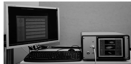
Figure 2. Photo of the electromagnetic system for nondestructive inspection of hollow axles.
