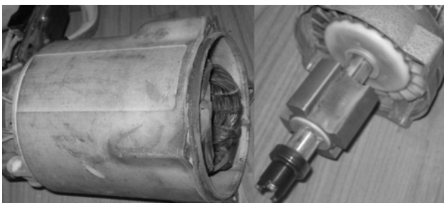
Fig. 3. A prototype of the new single-phase FRM
