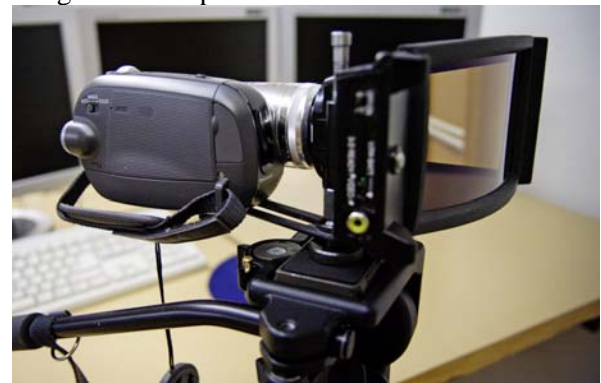
Fig.7: Time multiplexing system with a single camera at the UWB
