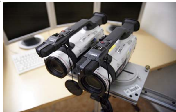
Fig.6: 3D setup with two cameras at the UWB
