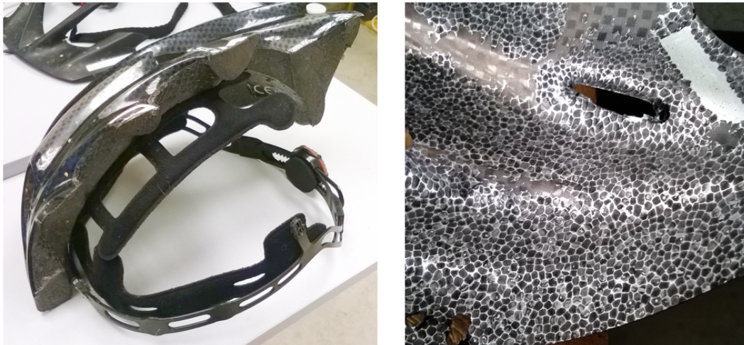
Figure 2.7: Analysis of in-molded cycling helmet produced by Limar. An adhesive connection of polystyrene cells and plastic liner can be seen on the right figure.
