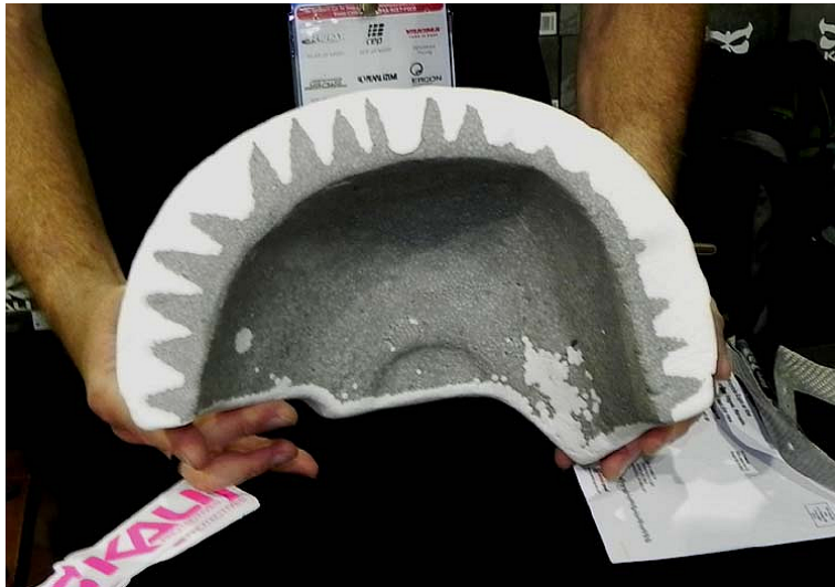
Figure 2.11: Double density liner produced by Kali [1].
