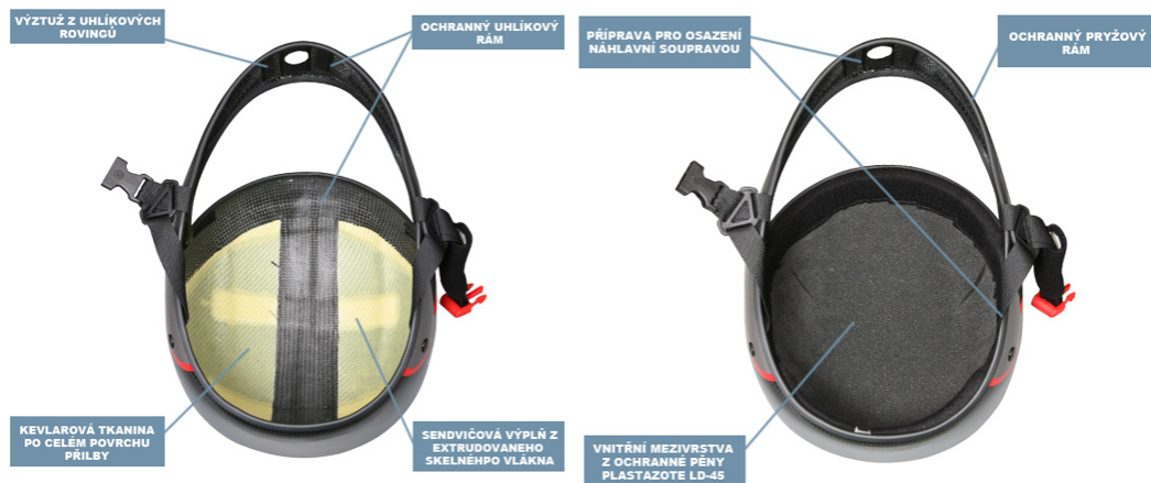
Figure 2.3: Typical hardshell helmet - a composite solution with the textile liner produced by Paraevoluce [2].
