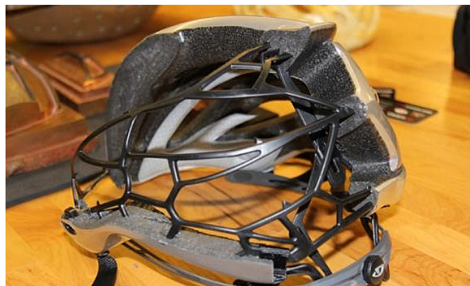
Figure 2.8: In-molded Giro helmet with inner plastic skeleton.
