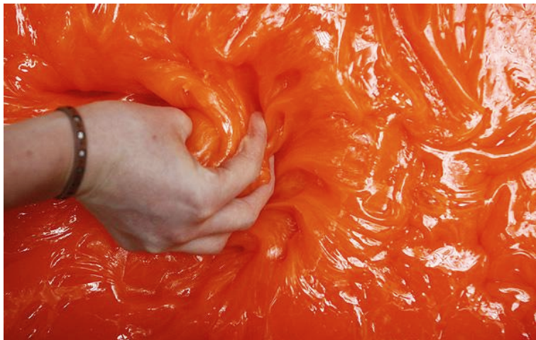
Figure 4.3: D3O in the original form before mixing with polymer [25].
