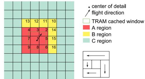
Figure 5: Loading order of RAM cache buffers.
