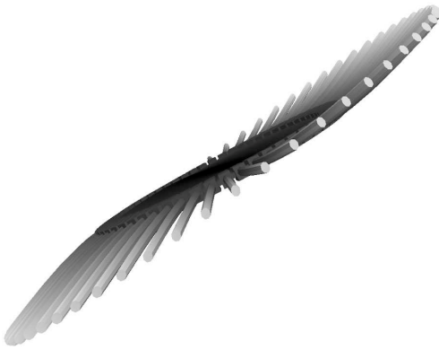
Fig. 6. Mode shape corresponding to eigenfrequency 69,5 Hz – 1 ND for non-rotating bladed disk
