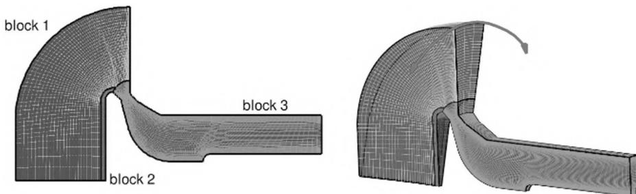
Fig. 3. Examples of structured multi-block grid, 2D – 3D
