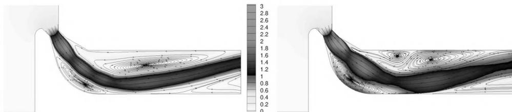
Fig. 6. Comparison 1<sup>st</sup> order solution (left), higher order solution (right), contours of Mach number, velocity streamlines
