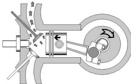
Fig. 1. Reciprocating engine at exhaustion phase, illustrative figure
