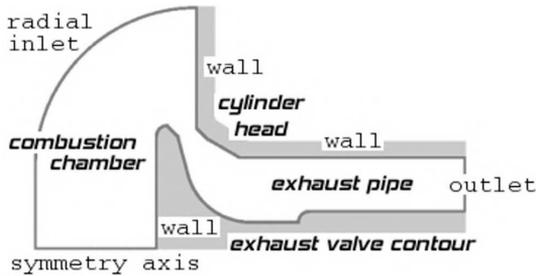
Fig. 2. Scheme of computational domain
