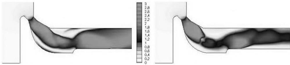
Fig. 9. Comparison of laminar (left) and turbulent (right) flow model, contours of Mach number
