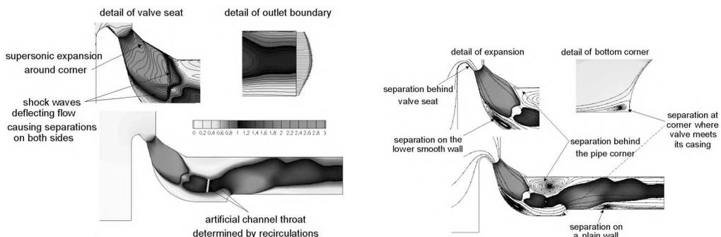
Fig. 10. Detailed flow structure of the turbulent solution
