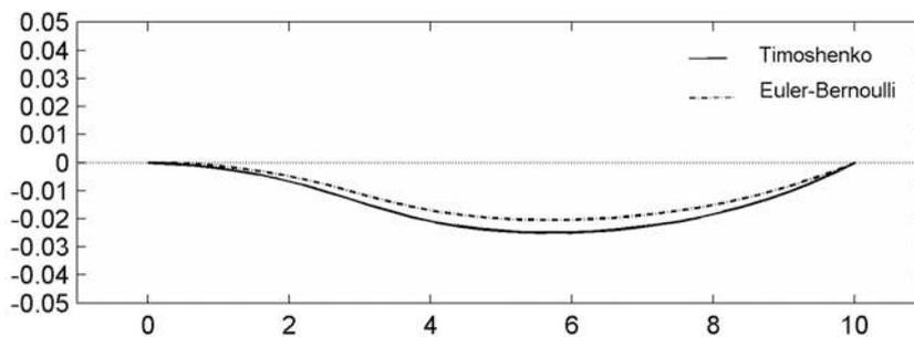
Fig. 2. A deflection of the optimal beam
