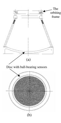
Figure 2. The omni-directional ball-bearing disc locomotion device; (a) Side view; (b) The surface of the OBDP
