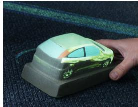
Figure 1. Typical foam model of a car (left) augmented by projection (right)
