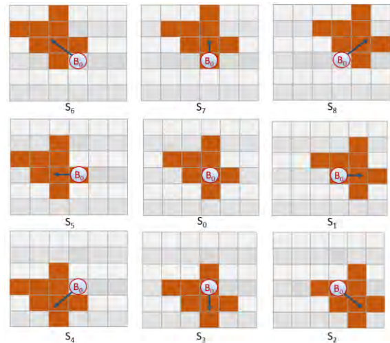
Figure 10. Nine similarity scores ( S_0 - S_8 ) calculation by shifting the indexed region of enrolled ear along different directions.
