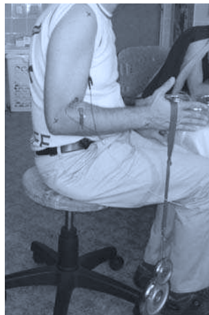
Fig. 1. EMG measurement, signal recording while carrying imposed load
