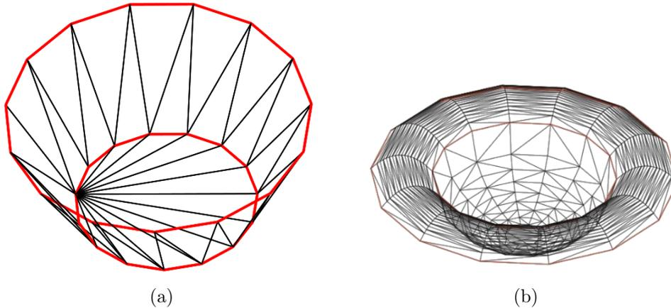
Figure 7.4: Two different inner parts. (a) Flat inner part. (b) Half-sphere ( $z = \sqrt{x^2 + y^2 - r^2}$ ) inner part.
