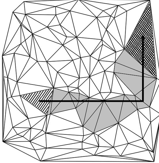
Figure 3.5: An example of the orthogonal walk. The search starts at the hatched triangle. Then it goes through all grey triangles. It ends in the cross-hatched triangle where the target point/triangle lies.
