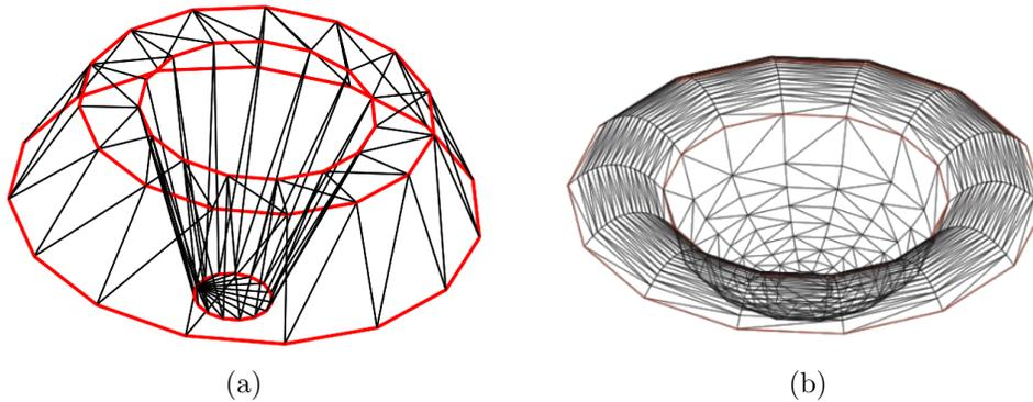
Figure 7.6: Two types of material extrusion. (a) Simple elevation extrusion. (b) Parabolic extrusion.
