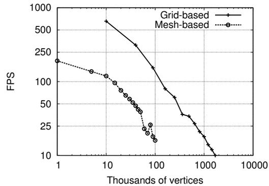
(b) FPS dependency on mesh/grid size (logarithmic scale, higher is better). Grid-based solution is faster when the detail is more or less the same.
