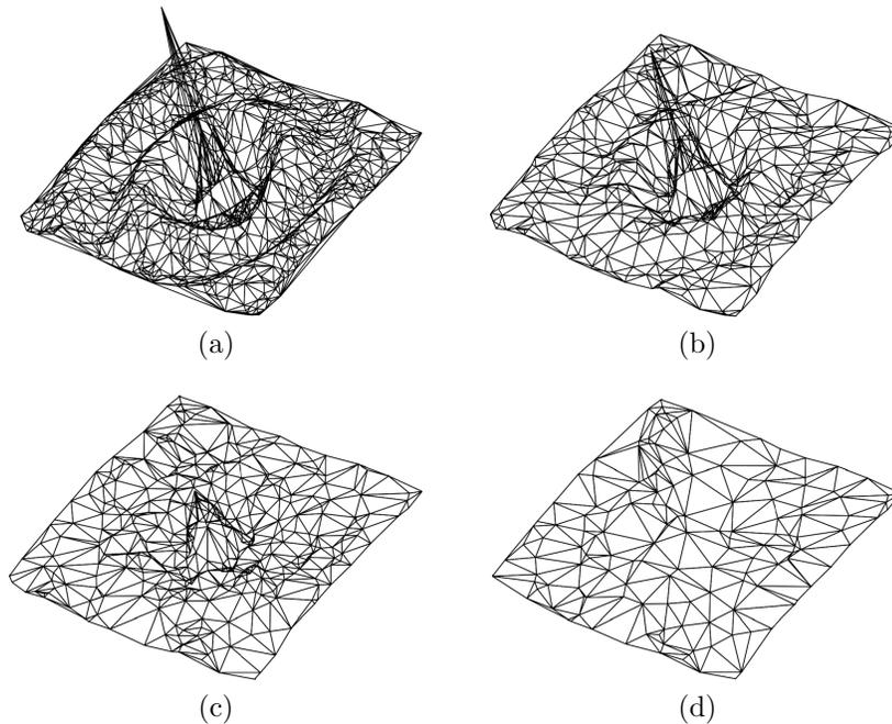
Figure 7.1: Four frames from the mesh simplification sequence, starting with the original mesh in (a) and ending with (d). Mesh is continuously being flattened by the erosion and simultaneously decimated.
