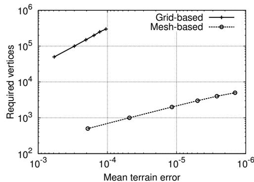
(e) Required vertices count for given detail (logarithmic scale, lower is better).
