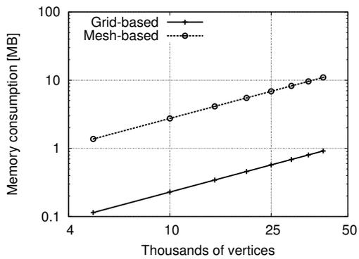
(c) Memory consumption comparison of grid-based solution and mesh-based method for uniformly distributed data (logarithmic scale, lower is better).
