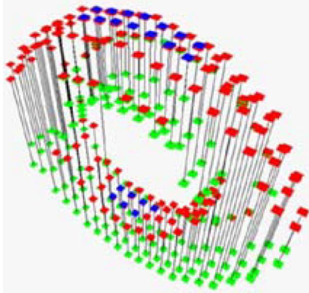
Figure 2.2: HS map of torus. Each red/green rectangle represents the upper/lower side of the height span, and each blue rectangle is for the upper limit of granular material on each height span [42].
