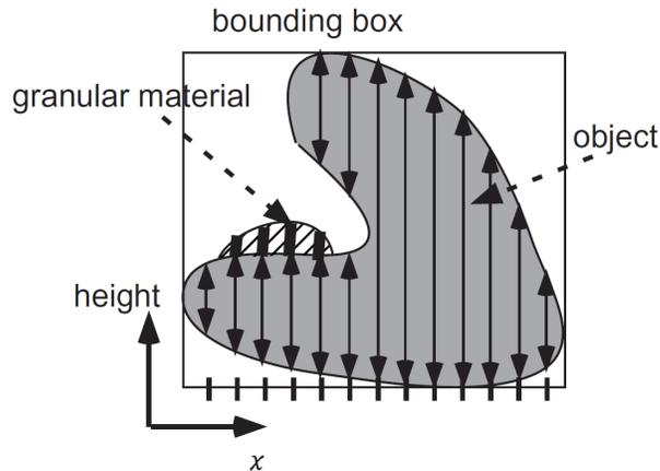
Figure 4.3: HS map example [42]. Each arrow represents a material mass in one span. Spans are stacked for each cell in the matrix. *Granular material* is represented as a particle system and it is independent of HS map.
