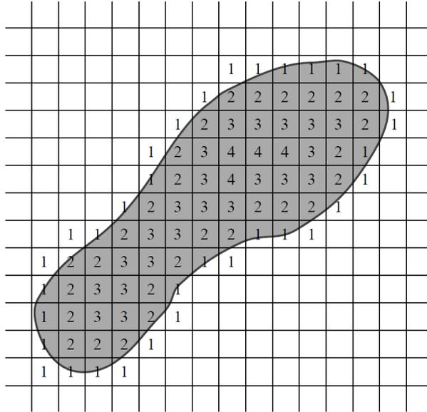
Figure 4.1: An example of virtual tool collision with the grid [60].
