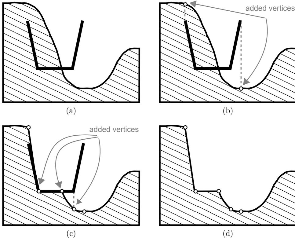
Figure 7.5: A simple tool imprinting sequence. Starting with (a) original terrain, thick edges represent the tool shape, (b) the outer part has been imprinted, (c) the inner part has been imprinted, (d) the terrain after imprinting of tool shape.
