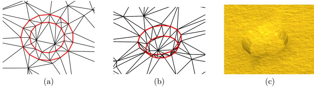
Figure 7.3: User tool footprint which compresses material. (a) Footprint view in a vertical projection. Wireframe model with thick lines indicating constrained edges. The enclosing circle represents the set of outer edges, inner circle the set of inner points. (b) Same as (a) but in isometric view. (c) Textured model. All models are displayed without erosion.
