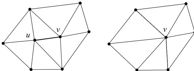
Figure 3.6: An example how an edge-collapsing algorithm works. Left: The edge  $uv$  will be collapsed. Right: The same mesh after collapsing  $uv$ . Only one inner vertex remains.
