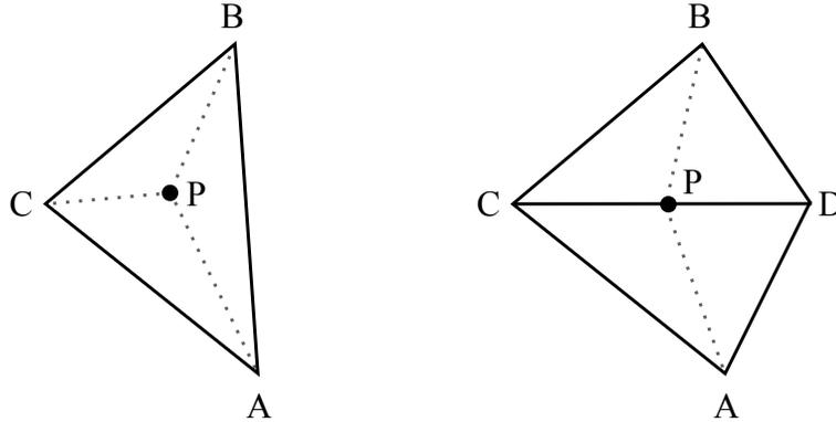
Figure 3.2: An example of triangle subdivision. Left: New point is inserted into the triangle  $ABC$ . Three new triangles are created. Right: New point is inserted on the edge  $CD$ . Both triangles must be subdivided. Four new triangles are created.
