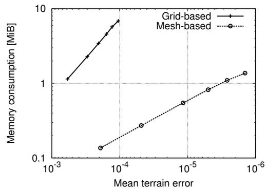
(d) Memory requirements of both methods for non-uniform terrain (logarithmic scale, lower is better).
