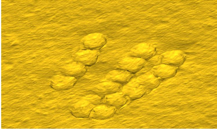
Figure 8.2: Separated eroded footprints of tool of half-sphere shape with parabolic material extrusion.
