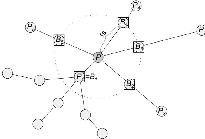
Figure 7.2: Material from the central vertex  $P$  will be moved to subdivision vertices  $B_k$ . Vertex  $P$  has neighbors  $P_i$ ,  $k = 1 \dots 5$ . Vertex  $P_1$  has the distance to  $P$  smaller than  $r_s$ . So a smaller amount of material will be relocated to it.
