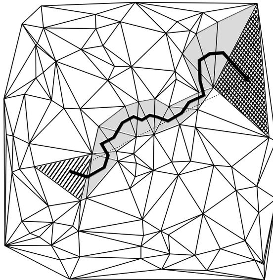
Figure 3.4: An example of the remembering stochastic walk. The search starts at the hatched triangle. Then it goes through all grey triangles in the direction of dotted line. It ends in the cross-hatched triangle where the target point/triangle lies.
