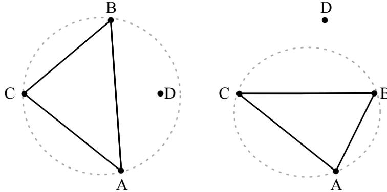
Figure 3.1: Delaunay circumcircle criterion. Left: Criterion is not met – point  $D$  lies in the circumcircle of triangle  $ABC$ . Right: Criterion is met.
