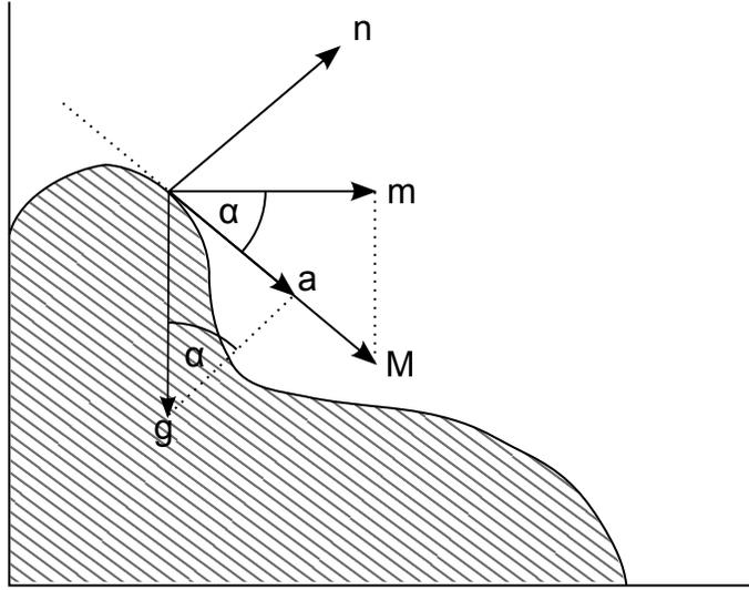
Figure 5.1: Relationship of all the vectors which are used for acceleration computation ( $a$ ).  $m$  is the orthogonal projection of the movement direction  $M = [M_x, M_y, M_z]$ .  $n$  is the normal vector to the surface and  $g$  is the standard gravity acceleration.
