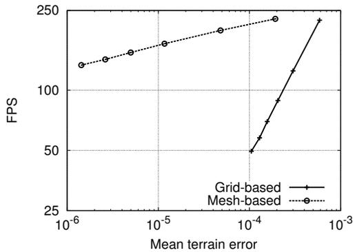
(a) FPS dependency on mean terrain approximation error (logarithmic scale, higher is better). Mesh-based solution is faster when there is a large difference in detail.
