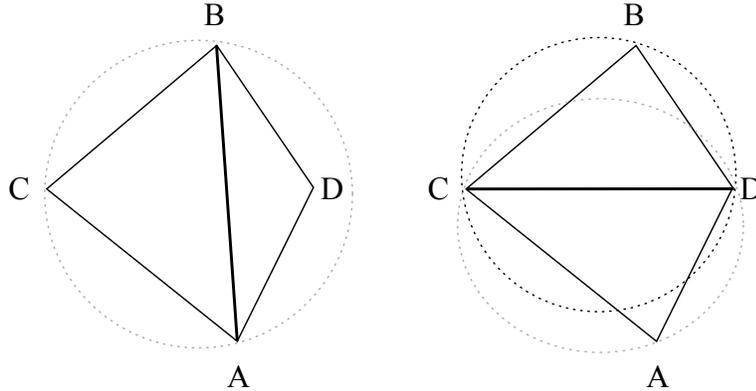
Figure 3.3: An example of the edge legalization for two triangles. Left: The configuration does not satisfy the empty circumcircle criterion, because the point  $D$  is inside of the circumcircle of the triangle  $ABC$ . Right: After the flipping of the edge shared by both triangles, the criterion is met for these triangles (both circumcircles of new triangles  $BCD$  and  $ADC$  are empty) and the check continues to the neighboring triangles.
