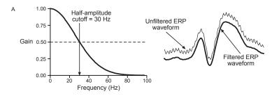
Figure 4.10: This figure illustrates the effects of low-pass filtering. The frequency response of the low-pass filter is on the left, the original P300 response and the low-pass-filtered response on the right. Although the filter deals with high-frequency distortions, it also decreases the amplitude of peaks and shifts their latencies. [6]
