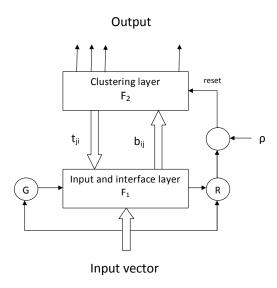
Figure 5.18: The simplified architecture of ART 2 network [44].
