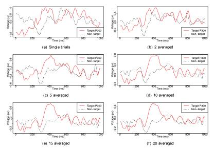
Figure 4.9: These figures show the effect of averaging trials together. For comparison, each figure depicts both target and non-target responses. [22]
