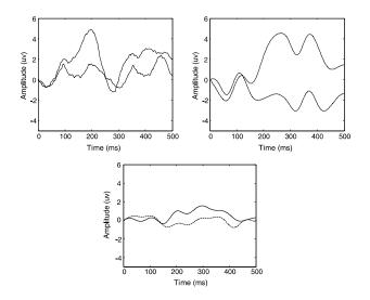
Figure 3.6: The P300 waveforms for different subjects. Only the subject whose response is in the top right figure has a strong P300. [9].
