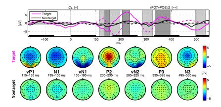
Figure 4.8: ERP components - spatial and temporal features. The upper plot shows averaged event-related potentials. Areas in gray correspond to the occurrence of ERP components. The lower part of the figure shows scalp maps representing spatial contribution of EEG channels related to the specific ERP components for both target and non-target responses. Note that for the P200 and the P300 components, the difference between target and non-target responses is the most significant. [18]
