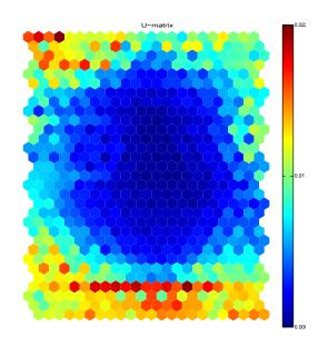
Figure 5.16: U-Matrix for the visualization of Self-organizing maps. The colors of the units represent Euclidean distances between the neighboring cluster units.
