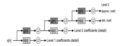
Figure 4.11: 3-Level Discrete Wavelet Transform
