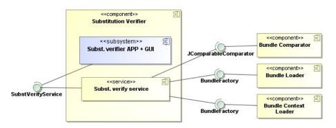
Figure 3: Architecture of the OSGi bundle compatibility verifier
