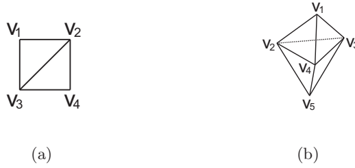
Figure 4.16: Each diamond is composed of two neighboring simplicial mesh cells, sharing a common face. Reference diamonds are depicted for 2D (a) and 3D (b) simulation mesh.
