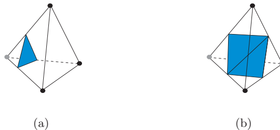
Figure 2.2: Marching tetrahedra. The two cases where triangulation is required, and the resulting triangulations. Case (b) can be rendered as a quadrilateral rather than two triangles, since the surface is guaranteed to be planar [51].
