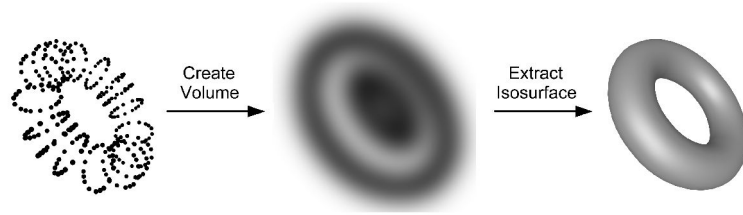
Figure 2.19: Overview of a volumetric algorithm.
