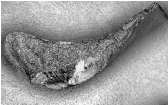
Fig. 10. Crack surface on the blade root
