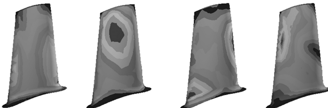
Fig. 2. Von Misses stress of the first four modal shapes
