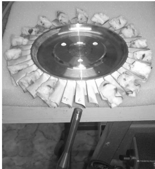
Fig. 6. Measuring system and the blisk with damped blades
