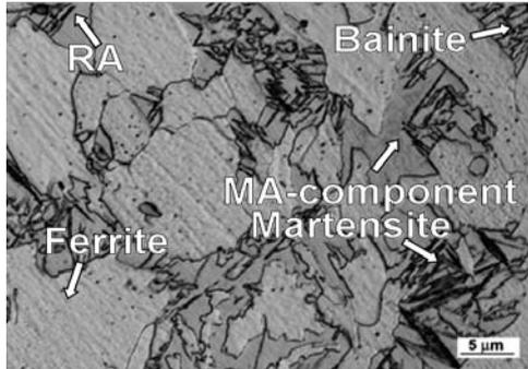
Fig. 3: Mixture of ferrite, bainite, martensite and RA, laser confocal microscopy, Nital
