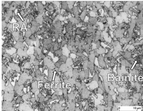
Fig. 1: Ferritic-bainitic structures with RA, light microscopy, two step etching: Nital + 10%Na<sub>2</sub>S<sub>2</sub>O<sub>5</sub>
