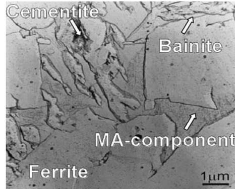
Fig. 2: Detail of bainitic formation and MA-component, transmission microscopy, Nital
