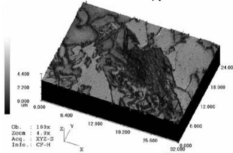
Fig. 4: 3D structure reconstruction, complex four phase structure, confocal laser microscopy
