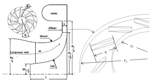
Fig. 1. Schematic of the centrifugal compressor stage geometry
