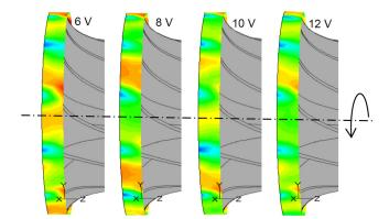
Fig. 10. Contours of meridional velocity at the impeller exit for four diffusers at design flow rate
