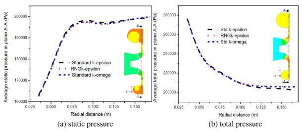
Fig. 5. Static and total pressure predicted with three RANS models
