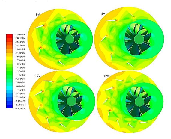
Fig. 14. Static pressure contours at design flow rate for four diffusers
