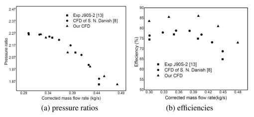
Fig. 6. Comparison of performances for vanless diffuser compressor
