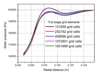
Fig. 4. Test of grid-solution independence
