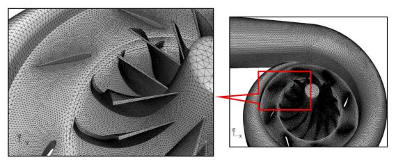
Fig. 3. Computational mesh of the vaned diffuser centrifugal compressor full sage
