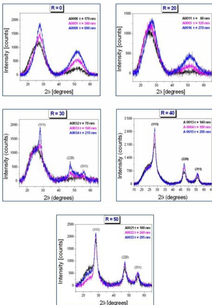
Figure 2 – Diffraction Patterns for Substance Sample Differing Thickness and Production
