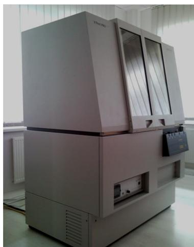
Figure 1 – PANalytical X’Pert PRO X-Ray Powder Diffractometer
