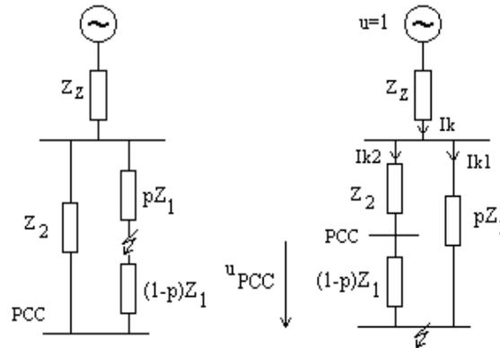
Figure 3 – Equivalent circuit for a looped network
