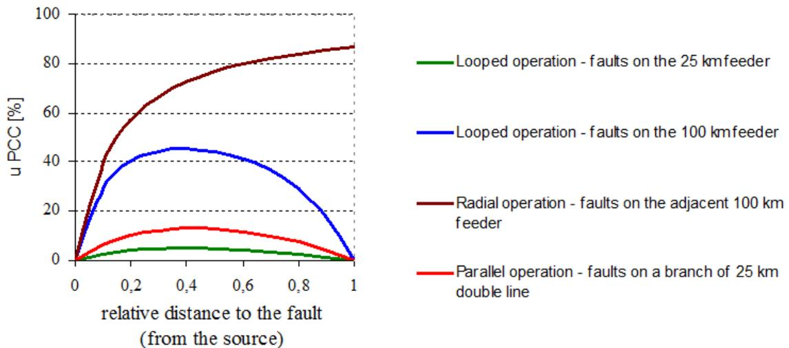
Figure 4 – Voltage at the PCC as a function of fault position on the feeders for various ways of network operation
