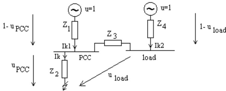
Figure 5 – Equivalent circuit for system with local generator
