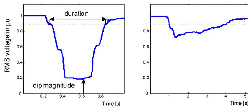
Figure 1 – Characteristics of a voltage dip caused by a) remote short-circuit fault and b) motor starting
