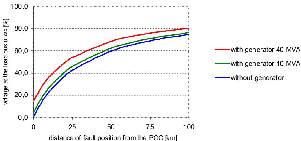
Figure 6 – Voltage at the load bus as a function of fault position for system with and without local generator
