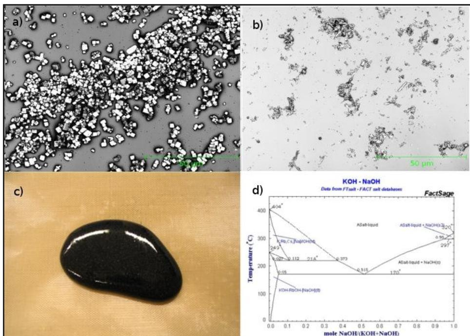
Figure 2 – a) PbTe cubes with laser confocal microscopy, b) CuS rods with laser confocal microscopy, d) Black PbS in eutectic hydroxides on Teflon foil, d) Eutectic diagram of NaOH and KOH
