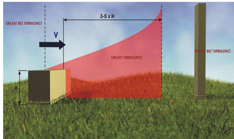
height, so rotor near the barrier must be placed higher in order not to be subjected to beats and vibration whereby financial demands of construction of the power plant body tube grow up. The influence of turbulence becomes weak with the growing distance from the barrier.
