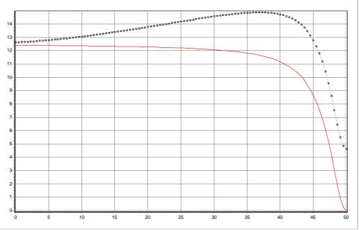
Fig.6: Power losses in conductive layer vs. rotor speed (SI units) for first mmf harmonic (solid line); total losses (dash-dotted line)
