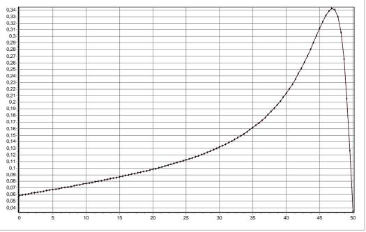
Fig.6: Torque calculated by means of both Maxwell and co-energy methods
