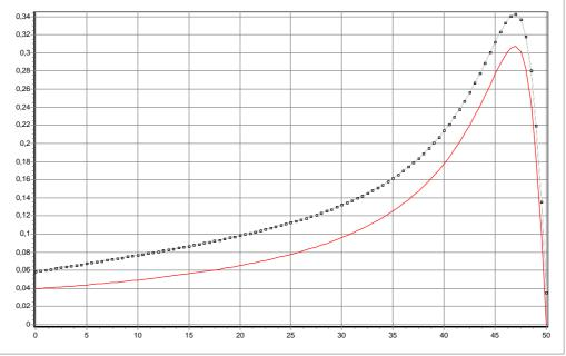
Fig.5: Torque-speed curves for first mmf space harmonic only - solid line, and for all considered mmf harmonics - dash-doted line, (SI units)
