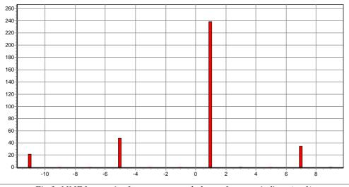
Fig.3: MMF harmonics for one separated phase of stator windings (p=1)
