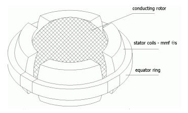
Fig.1: Spherical rotor - view
