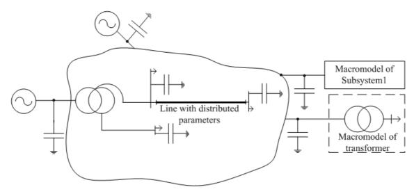
Fig. 2. Generalized scheme of electric system for transient research on the basis of mathematical models and macromodels
