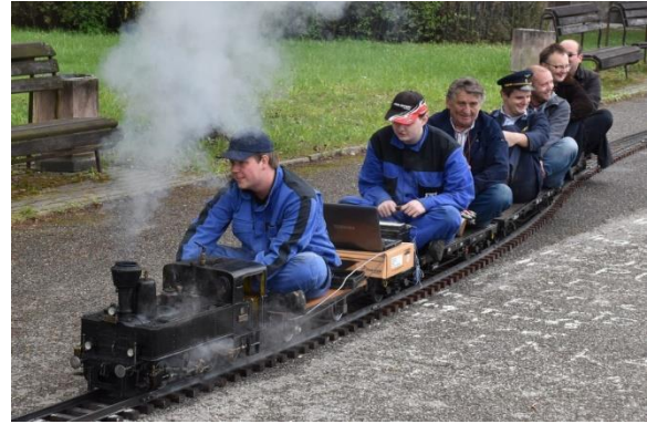
Fig 3. One of many measuring runs. A steam locomotive model 310.017 is pulling the MV-1 and three Pa-4 platform carriages with passengers.
