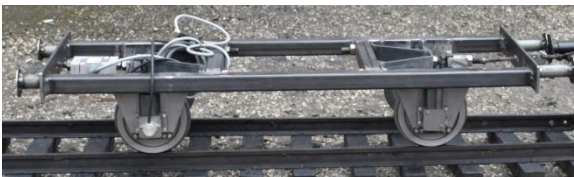
Fig 2. Detail of MV-1 under construction. The strain gauge and encoder can be seen on the left side.
