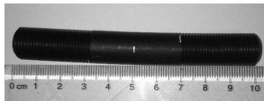
Figure 2: Photo of the CRB specimen manufactured from the pipe wall. The specimen is noticeably deformed.
