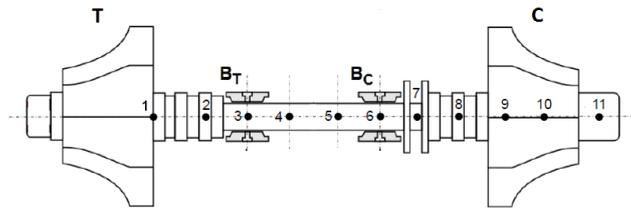
**Figure 1:** Turbocharger rotor-bearing system scheme.
