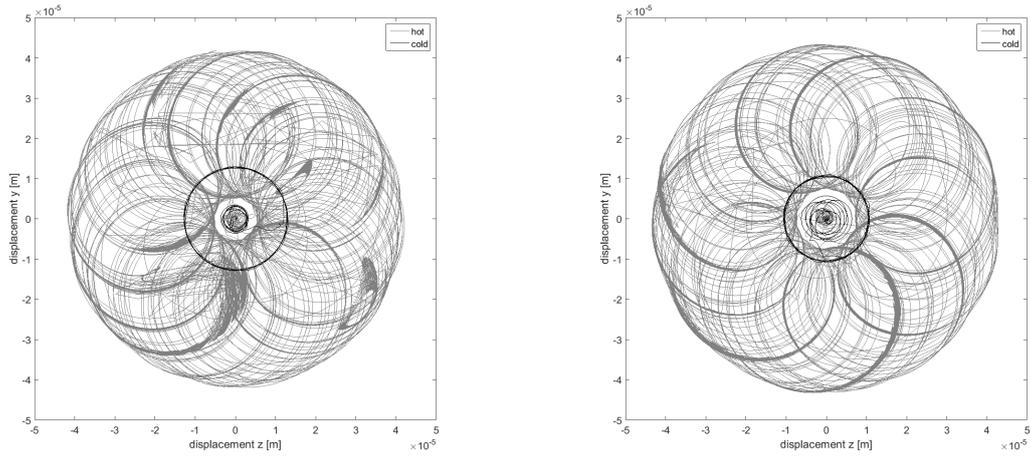
**Figure 2:** The orbits of journal centers of bearing  $B_T$  (on the left) and  $B_C$  (on the right) for rotational speed 100 krpm.
