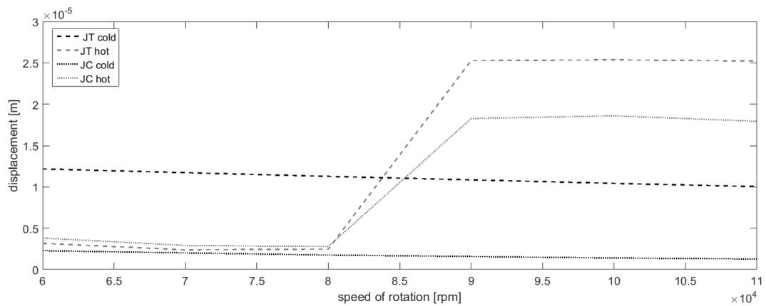
**Figure 4:** Dependence of maximal displacement magnitude of the journal centers.
