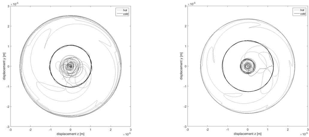
**Figure 3:** The orbits of floating ring centers of bearing  $B_T$  (on the left) and  $B_C$  (on the right) for rotational speed 100 krpm.
