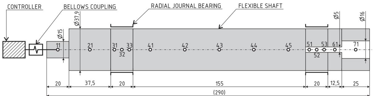
**Figure 1:** Geometry of the sample shaft.
