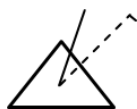
Figure 9. Proposed (SAR) aircraft glyph which can be distinguished from the active target glyph shown in Fig. 1(b) since no rotation is used. COG might be indicated by a solid line, if available.
