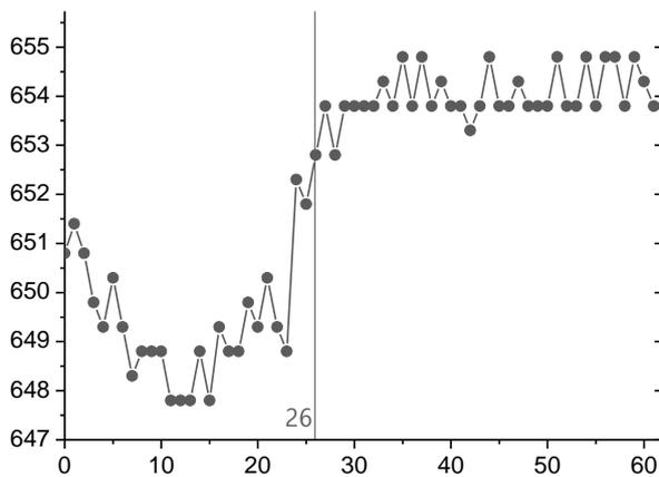
Fig. 2: Etched AlN micromechanical cantilever on a Si substrate with indication of the direction and of the number of steps in Raman scanning analysis (top figure). Variation of the centre of the  $E_2$  Raman band of AlN due to the presence of mechanical stress in dependence on the position of the focused laser beam (bottom figure).
