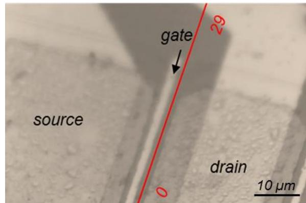
Fig. 1: Optical micrograph showing the channel of the HEMT with indication of the direction and number of steps during Raman scanning analysis (30 steps).
