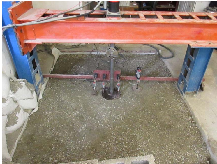
Figure 3. Prepared test box before starting loading
