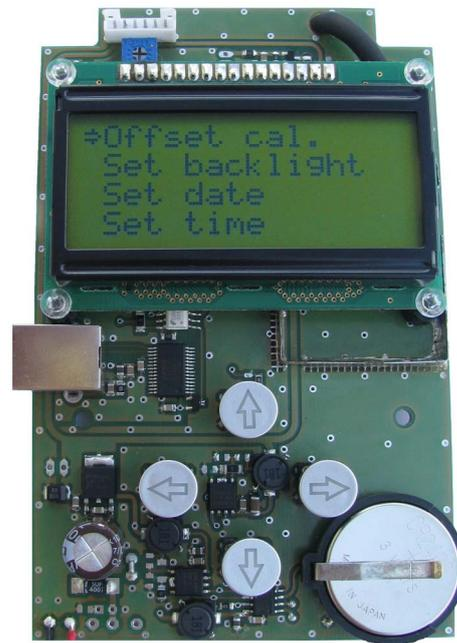
Figure 6. Shouldered printed circuit board of HK-01 Data Logger luxmeter
