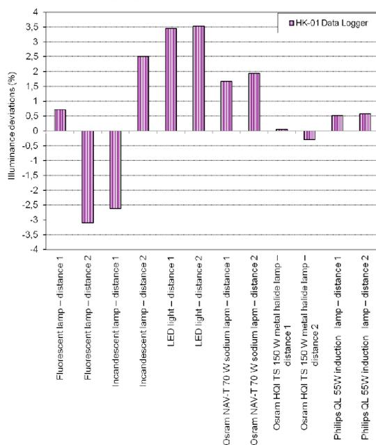
Figure 5. Response of the light sensors to the light of different light sources, with illuminance deviations expressed in percent values.
