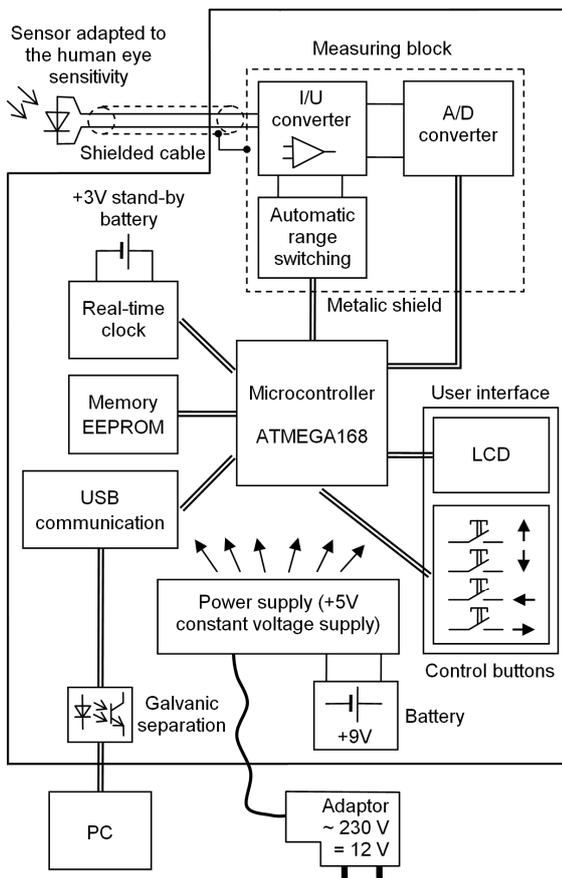
Figure 1. Block diagram of luxmeter connection.
