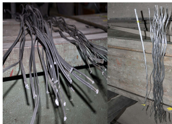
Figure 1. Tested samples : left - ACSR cable, right - ground cable
