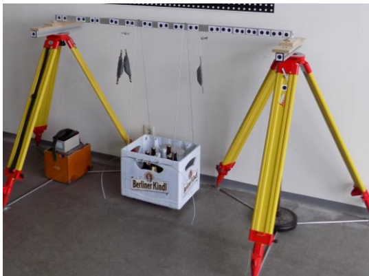
Fig. 1. A six-point bending test apparatus for an aluminium beam specimen.
