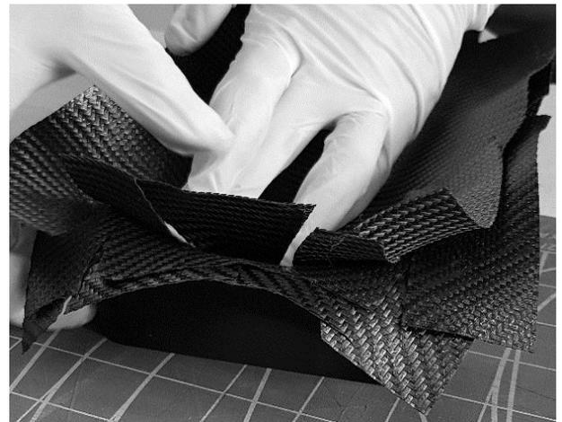
Fig. 1. Placing composite layers in mold.
