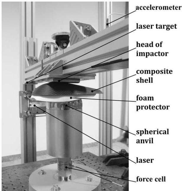
Fig. 2. Impact test.
