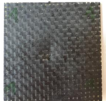
Fig. 2. Impact loaded surface of a sample loaded with 3 J energy.
