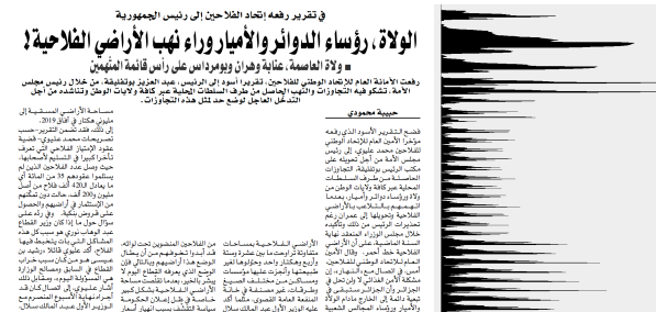
Figure 2: The input image with a plot of the horizontal projection profile on the right.
