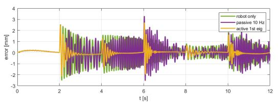
Fig. 3. Vibrational response of end-effector to force impulses on trajectory
